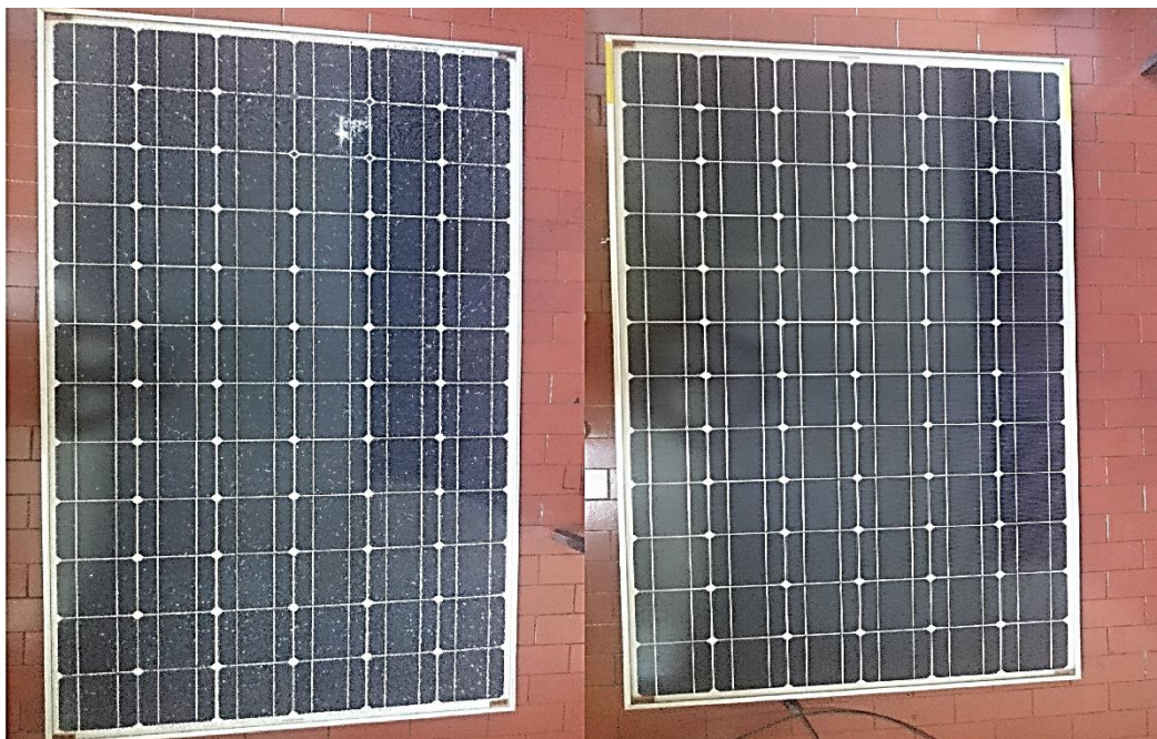
Figure 3.1 - The two panels tested in the laboratory: left side (broken glass and a broken cell), right side (healthy panel)
